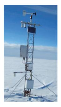
Fig. 2. Kominko-Slade station prior to servicing. Instrumentation consists of a Weed platinum resistance thermometer (PRT), a two-junction thermocouple temperature-difference sensor set (measuring temperature difference between the sensor boom at top of the tower and at the half meter mark above the snow), an R.M. Young Wind Monitor, a Vaisala HMP 45 for humidity, and a Paroscientific pressure sensor within the enclosure.
