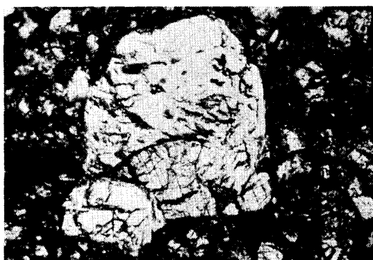
e. Lithic fragment in which a pyroxene with coarse exsolution lamellae is in contact with plagioclase by a smoothly curved boundary.
