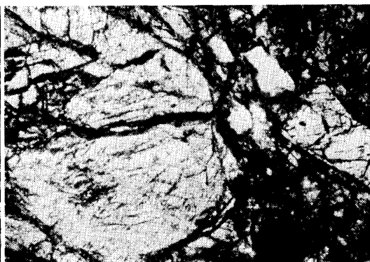
f. Large pyroxene fragment with nearly uniform Mg-rich composition but with no exsolution lamellae.
