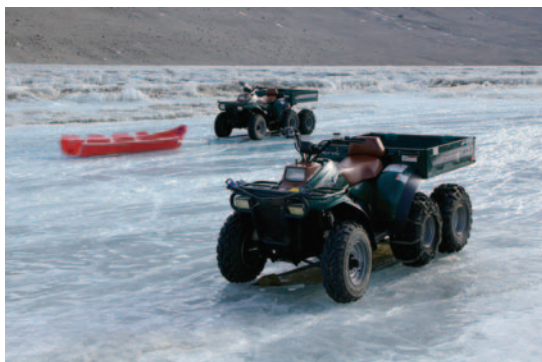
図 3 湖氷上に駐車中のバギーと車体下のオイル受け Fig. 3. Buggies parking on lake ice with oil pans under the bodies.
