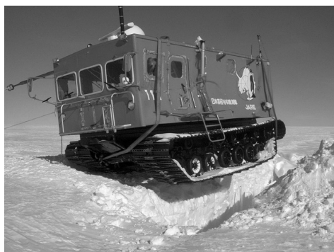
図 11 引き上げ時の雪上車前方及び後方 Fig. 11. Snow vehicle over the crevasse, supported by two other snow vehicles.
