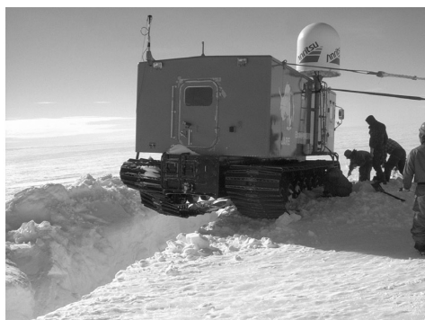
図 11 引き上げ時の雪上車前方及び後方 Fig. 11. Snow vehicle over the crevasse, supported by two other snow vehicles.
