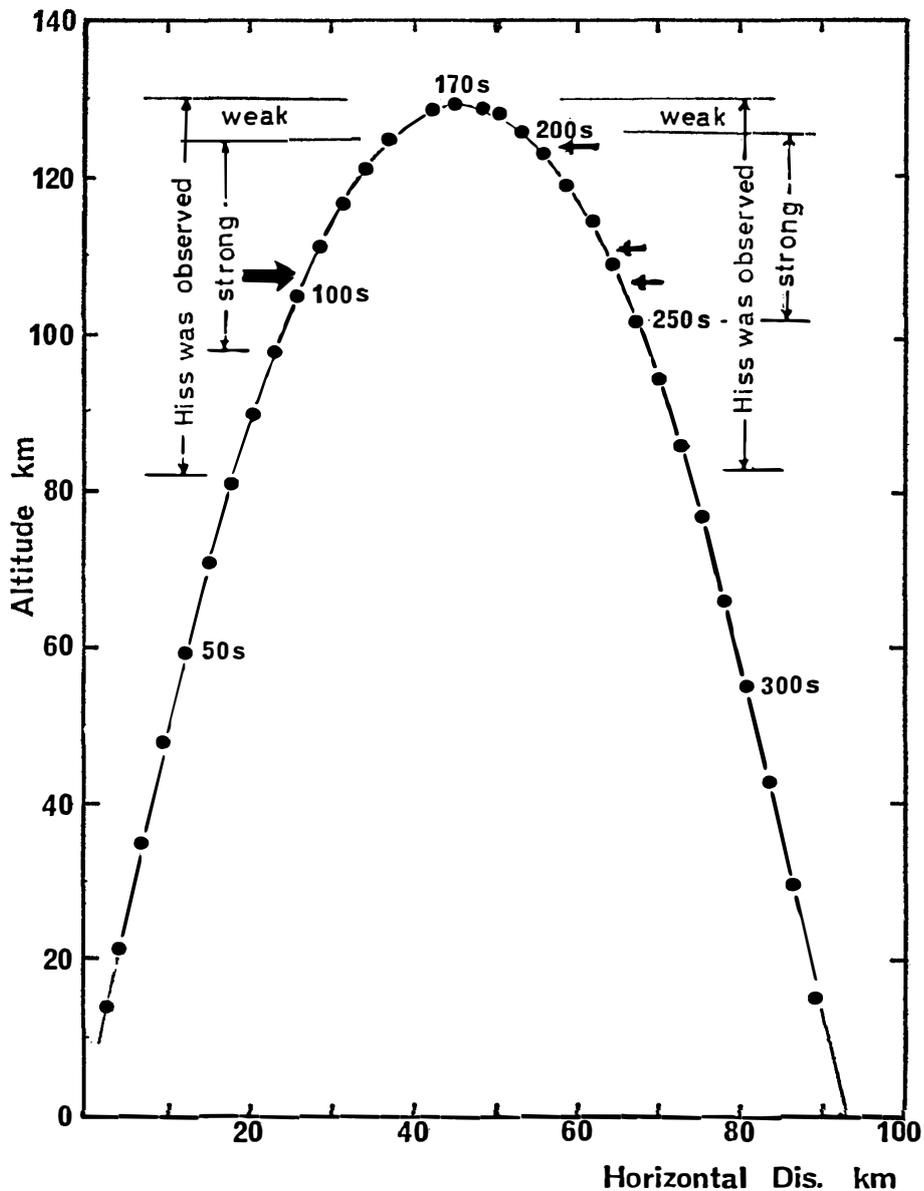
Fig. 11. An aspect of the position where hiss was observed on the trajectory of S-210JA-19.
