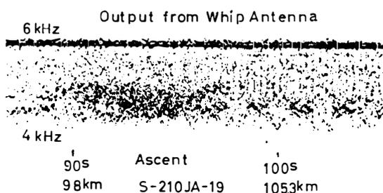
Fig. 10. The frequency vs. time spectrum for the whip antenna output of the VLF wide-band receiver.
