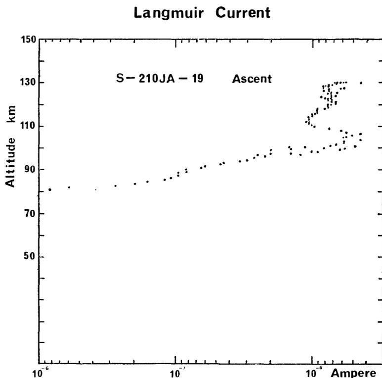
Fig. 1. The profile of the Langmuir probe current with altitude during the ascent.
