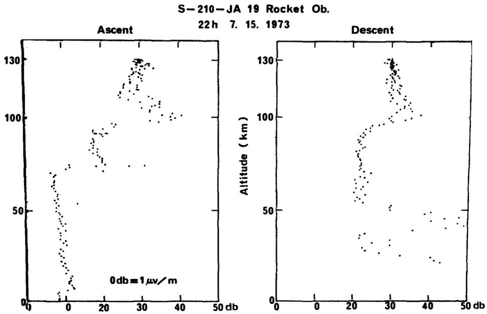
Fig. 3. The profile of the field intensity at 30 kHz with altitude.
