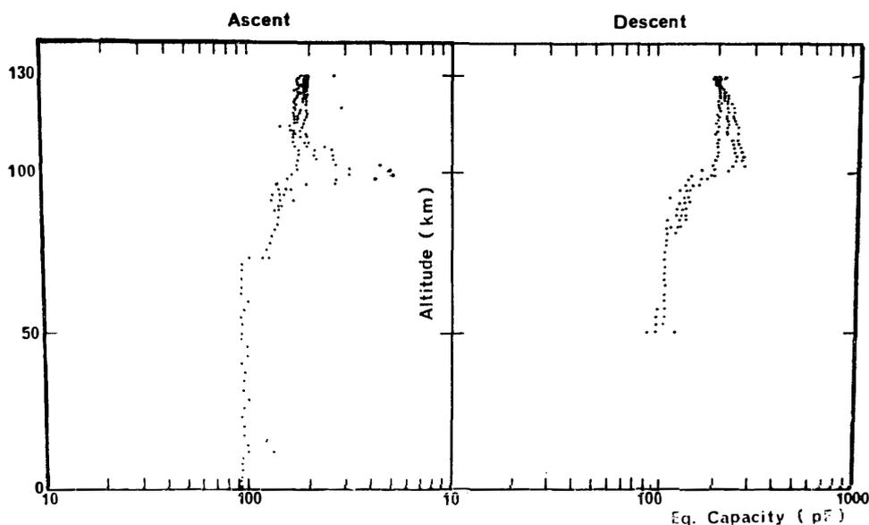
Fig. 4. The profile of the equivalent capacity of a whip antenna at 17.5 kHz in the ionosphere.
