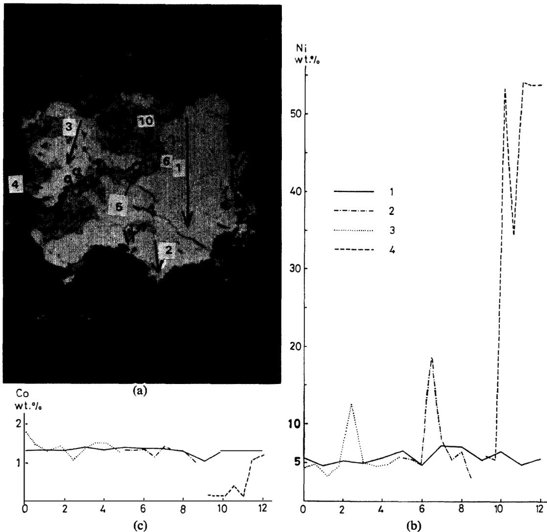
Fig. 5. Photograph and analytical traverses of a metal grain in the Yamato-7307 howardite. The size of the grain is  $0.46 \times 0.41$  mm. The horizontal scale 12 corresponds to 0.24 mm.
