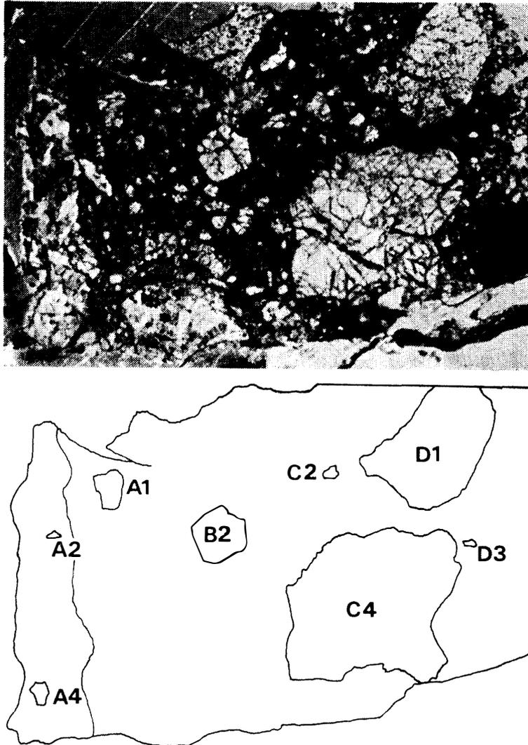
Fig. 1. Photograph and map of thick-section No. 14 of Yamato-7307 howardite. Width is 5 mm.
