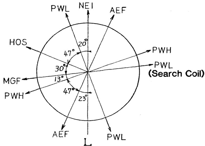
Fig. 3. Orientation diagram of sensors and antennas of the S-310JA-11 and -12 rockets.
