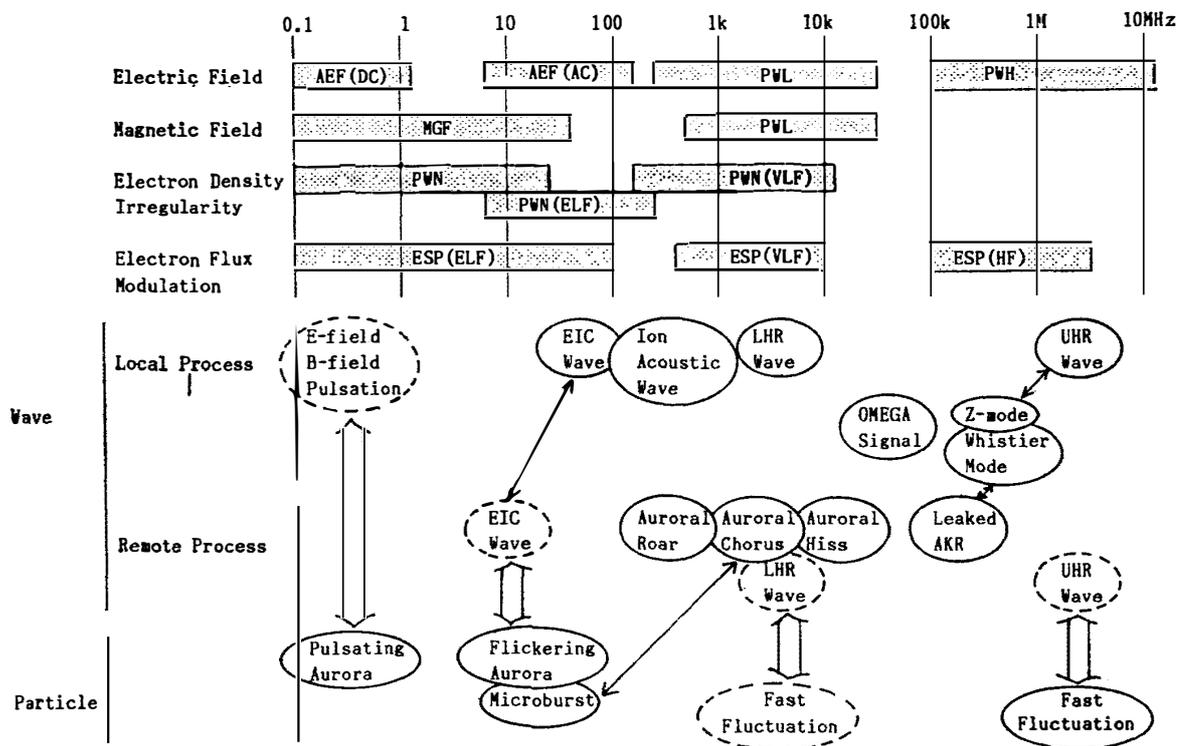
Fig. 1. Frequency ranges covered by the instruments on board the S-310JA-11 and -12 rockets, and wave-particle interaction processes to be measured by these instruments.
