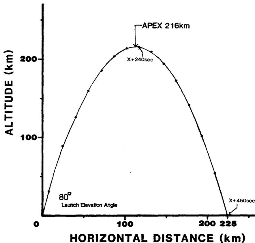
Fig. 4. Calculated flight trajectory of the S-310JA-11 and -12 rockets.
