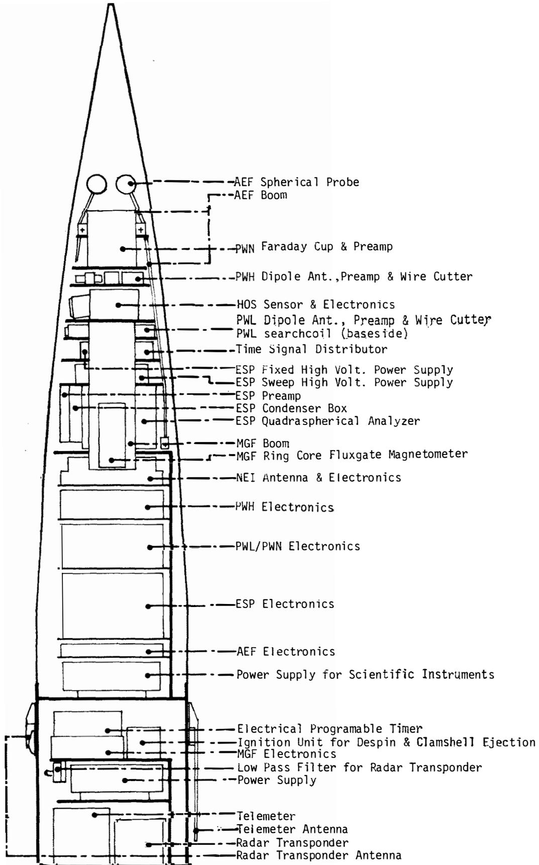
Fig. 2. Payload configuration of the S-310JA-11 and -12 rockets
