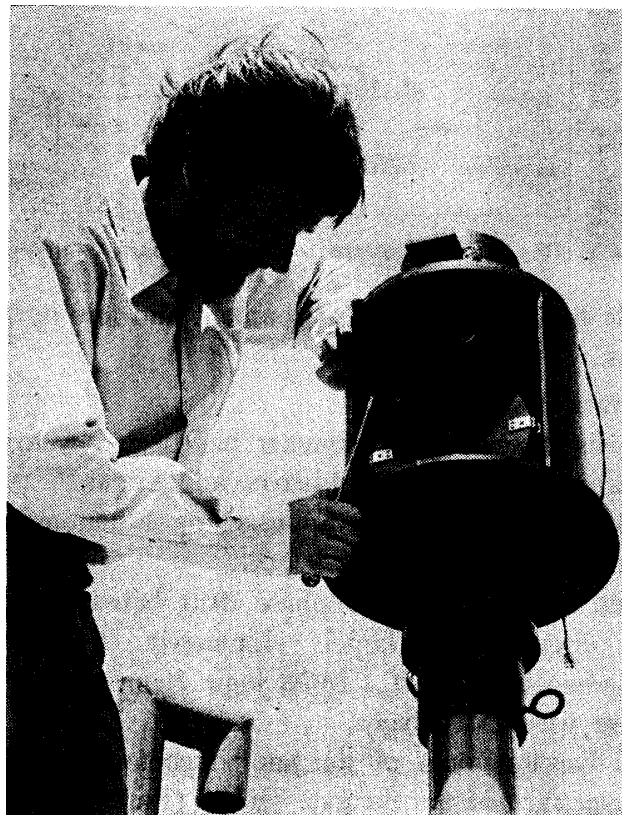
Fig. 11. Auroral all sky camera (Exterior cover removed).
