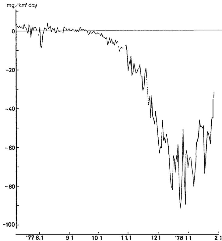
Fig. 2. Daily amounts of condensation and sublimation obtained by the atmometer method, July 7, 1977–January 31, 1978.
