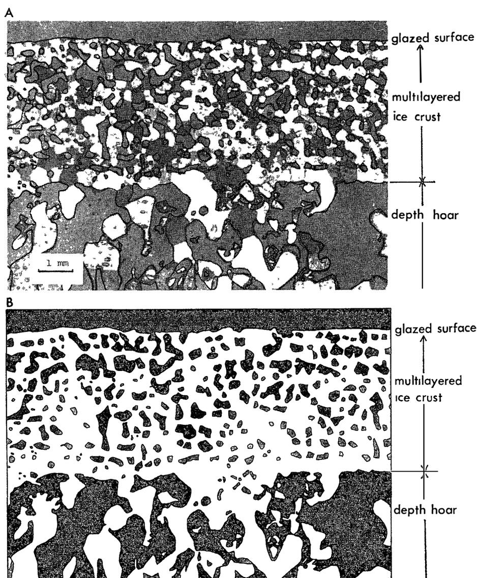
Fig. 6 A. Microphotograph of thin section of surface snow layer with multilayered ice crust in crossed polarized light. B. Sketch of the microphotograph showing the snow particles and vacant spaces in white and black respectively
