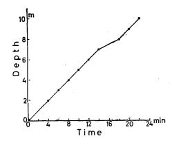
Fig. 3. Drilling rate for the firn at Mizuho Plateau. Station, H101; Elevation, 1309 m; Date, 11 November 1973; Air temperature, -17.5°C; Wind speed, 9 m/s; 10 m snow temperature, -20.1°C.
