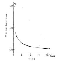
Fig. 4. The 10 m snow temperature versus the time which has elapsed after the end of drilling at Mizuho Plateau. Station, C98; Elevation, 1820 m; Date, 21–22 November 1973.
