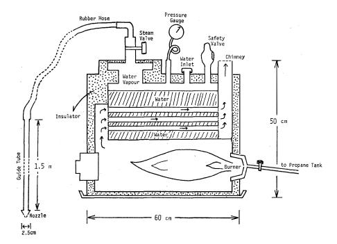
Fig. 1. A schematic drawing of the steam drill. The rubber hose, the burner and the pressure gauge are detached during the transportation on a sledge.
