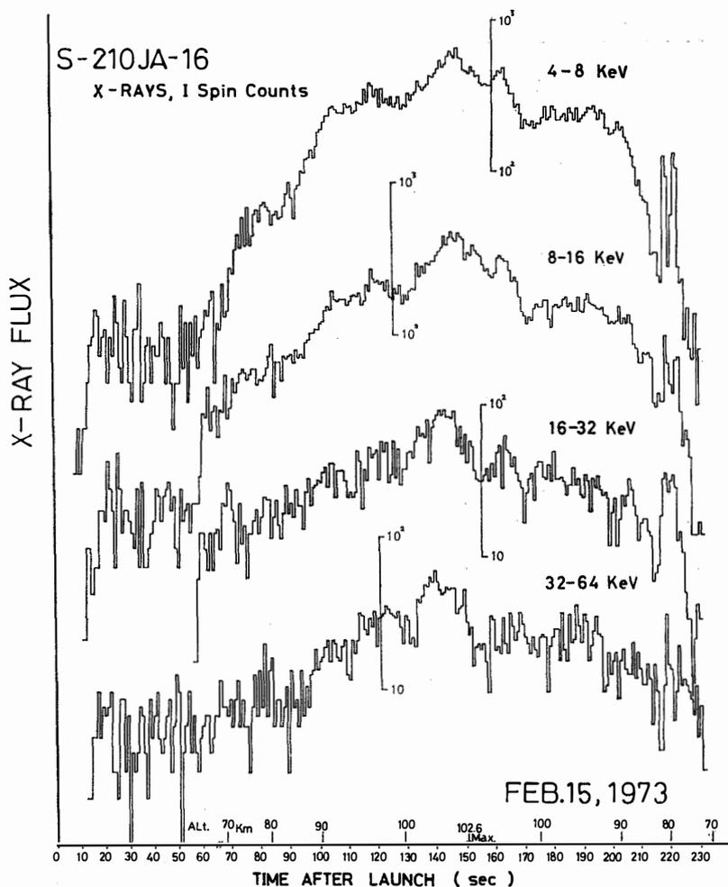
Fig. 7. Time profiles of X-ray intensities measured in four channels having different energy ranges aboard the S-210JA-16 rocket, where the X-ray counts are given every spin cycle.
