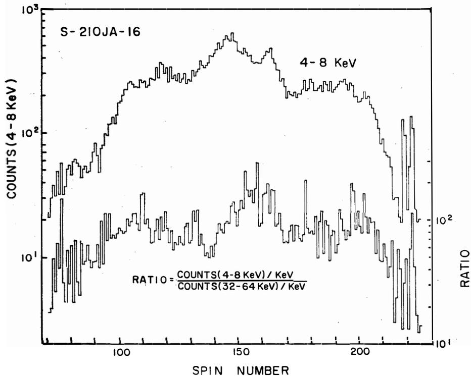
Fig. 8. Time variations of X-ray intensities in the 4-8 keV energy range and of the ratio of the counts from the 4-8 keV channel to that from the 32-64 keV channel.
