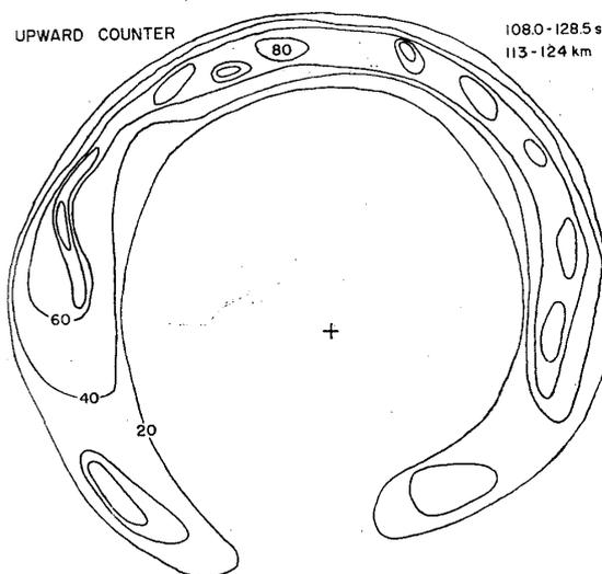
Fig. 2. An example of all-sky contour maps of X-ray intensity taken by a S-210JA-3 rocket during a precession cycle. Attached figures give counts per 1/20 s. A gap appeared below in the whole circle is almost in the geomagnetic south direction. A cross mark in the center indicates the direction of the rocket precession axis, being  $16^\circ$  from the zenith.
