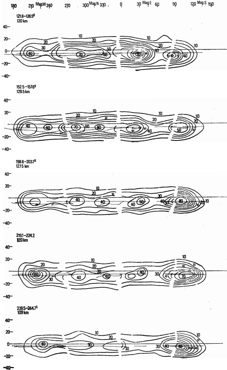
Fig. 3. Some examples of isophoto maps of X-ray fluxes viewed from an altitude between 120 km and 109 km in the descent of the S-210JA-3 rocket. Numerical units are the same as those in Fig. 2. Dotted lines indicate the location of the brightest arcs of optical aurora.
