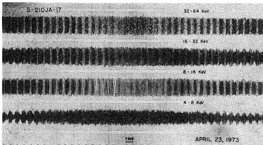
*Fig. 10. Reproduction of the pen-writing recording chart of X-rays obtained in the S-210JA-17 rocket experiment. Patterns from four different energy channels are displayed, respectively. One cycle up and down in each diagram equals 32 counts of X-rays. Periodic reduction in amplitude seen from the lowest pattern are attributed to over-sensitivity of the pen-writing recorder due to very high counting rates observed.*
