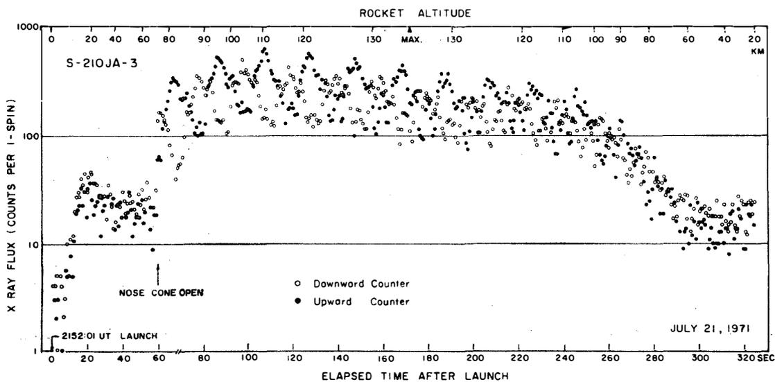
Fig. 1. Time profiles of X-ray intensities measured aboard the S-210JA-3 rocket, where counts per spin cycle are plotted. Open and solid circles correspond to the upward- and the downward-directed detectors, respectively.
