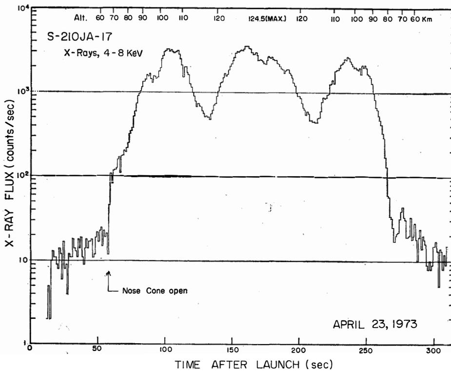
Fig. 9. The entire time profile of 1-s counts of the 4-8 keV X-rays observed aboard the S-210JA-17 rocket.
