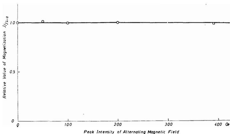
Fig. 2. Change in the intensity of stable remanent magnetization with the demagnetization by alternating magnetic field.
