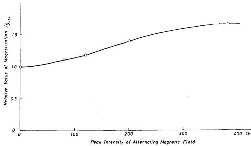
Fig. 4. Change in the intensity of remanent magnetization with the demagnetization by alternating magnetic field.
