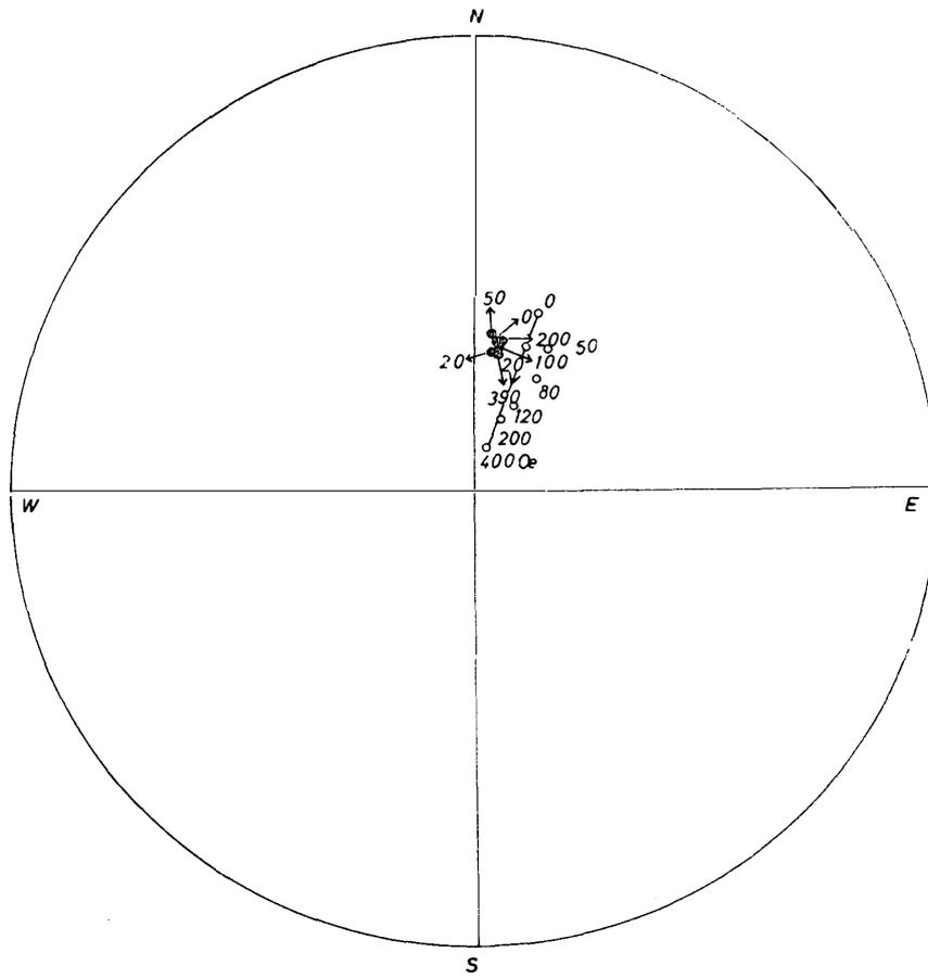
Fig. 3. Change in the direction of remanent magnetization with the demagnetization by alternating magnetic field.
