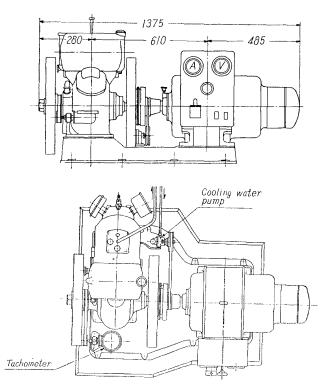
Fig. 28. Yammar K-6 type, 3 KVA Diesel electric generator (100 V, 3φ) (presented by Yammar Diesel Co.).
