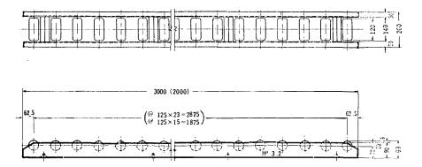
Fig. 19. NE-125 type roller conveyer.
