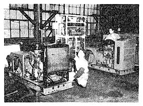
Fig. 31. Improved type 20 KVA (100 V,  $3\phi$ ) electric generators and their control panel (prepared by Isuzu Auto. Co. and Meidensha).
