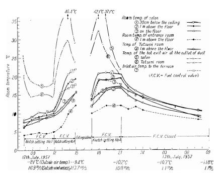
Fig. 38 (b). Temperature change in living hut (heated by oil only, thermostat 1.25 (18°C)).
