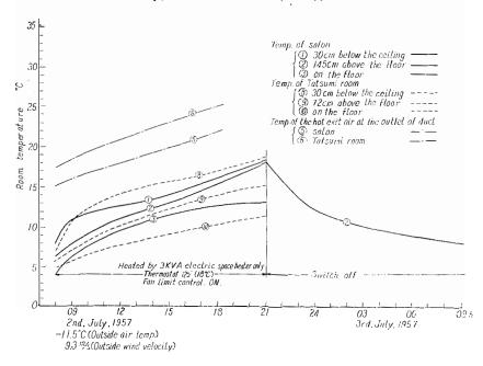
Fig. 38 (c). Temperature change in living hut (heated by 3 KVA electric space heater only, thermostat 1.25 (18°C)).
