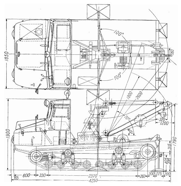
Fig. 4. KC 20-3 R type snow-wrecker made by the Komatsu Manufacturing Co. (The first expedition, 1956/58).
