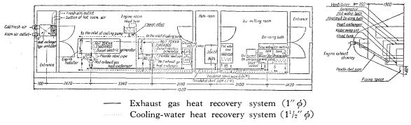
Fig. 40. Engine room and cold and hot water making system utilizing waste heat of 40 IP Diesel engines (prepared in the factory of the Nihon Univ. for the first expedition).
