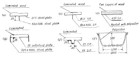
Fig. 13. Sliding plane of runner of snow sleighs (see Table 4).
