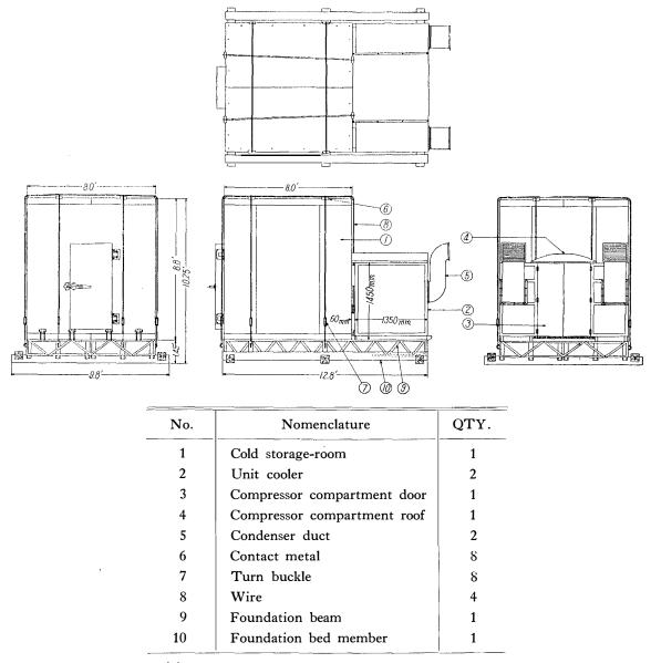
Fig. 50 (a). Cold storage-room prepared for the second expedition (made by the Nakano Refrigerating-Machine Co.).
