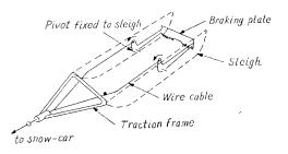
Fig. 14. (a) Principle of the automatic brake prepared for the wooden sleighs (manufactured by Yokohama Yacht Co.).
