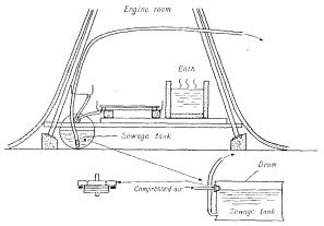
Fig. 45. Sewer system in the engine room at the Syowa Base.
