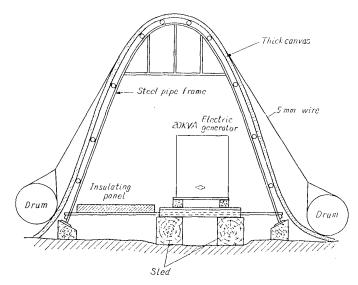
Fig. 44. Section of engine room.
