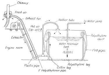
Fig. 48. Water reservoir tank.
