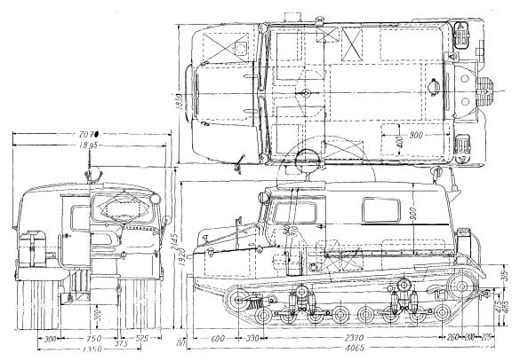
Fig. 7. New KC 20-3 S type "Ginrei" gasoline snow-car made by Komatsu Manufacturing Co. (The second expedition 1957/58).
