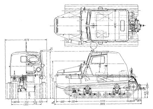
Fig. 8. New KD 20-2T type "Ginrei" Diesel snow-car with torqueconverter made by Komatsu Manufacturing Co. (The second expedition, 1957/58).
