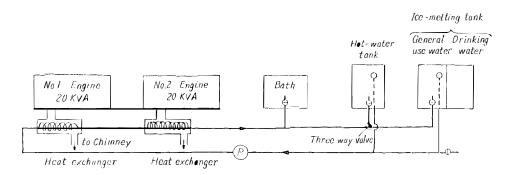
Fig. 43. Simplified water making system installed in the engine room of the Syowa Base.
