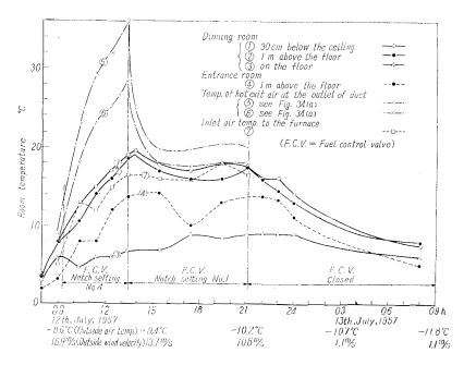
Fig. 38 (a). Temperature change in main hut (heated by oil only, thermostat 1.25 (about 18°C)). The index numbers in this figure correspond to the one shown in Fig. 34 (a).
