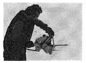
Fig. 52. Ice-saw driven by a small 2-cycle gasoline engine (prepared by the Fuji Heavy Industry Co.).
