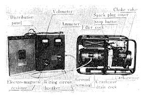
Fig. 56. Portable 1 KW, A. C. 100 V electric generator (prepared by Tokyo Engine Ltd. Co.).
