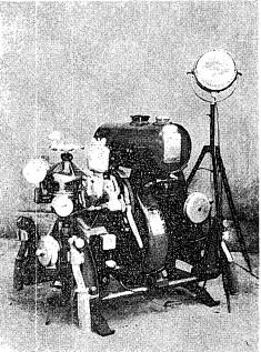
Fig. 58. Water pump driven by a 5hp, 2-cycle gasoline engine (prepared by the Tokyo Engine Co.).
