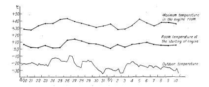
Fig. 29. Engine room temperature and atmospheric temperature in the winter at the Syowa Base (Aug. 20th to Oct. 10th, 1957).Room temperature was measured at 1.2 m above floor.
