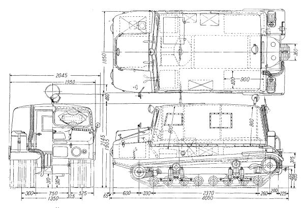
Fig. 3. "Ginrei" KC 20-3 S type snow-car made by Komatsu Manufacturing Co. (The first expedition, 1956/58).
