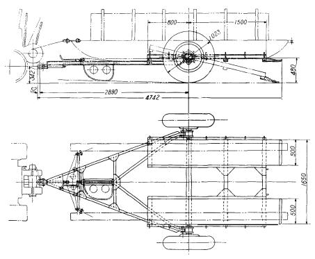
Fig. 24. Trailer for transporting a loaded sleigh on the rock zone.
