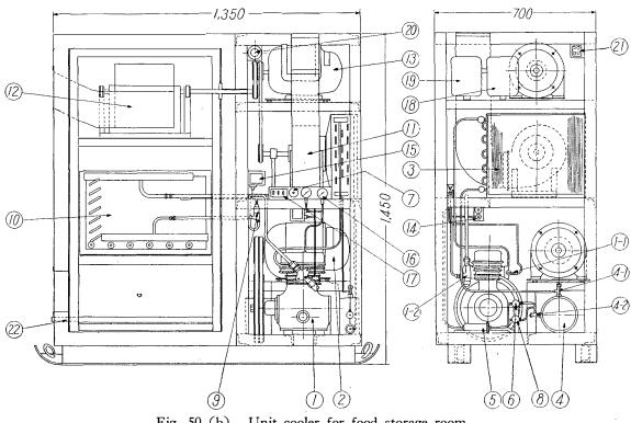
Fig. 50 (b). Unit cooler for food storage room (made by the Nakano Refrigerating-Machine Co.).
