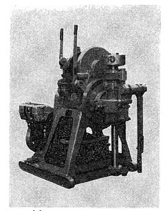
Fig. 53 (a). T-100 type boring machine (prepared by the Tone Boring Machine Co.) driven by a 4-cycle gasoline engine (prepared by the Fuji Heavy Industry Co.).
