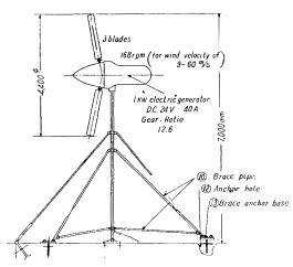
Fig. 51. Wind-mill for 1KW electric generator (constructed & presented by Honda Giken Kogyo Co.).
