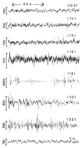
Fig. 1. Noise signals at various wind velocities. Numerals in parentheses mean the wind velocity (in m/s). The amplitude scale (in  $\mu cm/s$ ) is indicated on the left of each noise. t. n. means the tape-out noise including the electric noise generated in a data recorder and its amplitude is calculated in terms of ground velocity.
