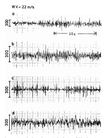
Fig. 5. Noise signals at various depths under a wind velocity of 22 m/s. d is recorded at a depth of 10 m. See caption of Fig. 3.
