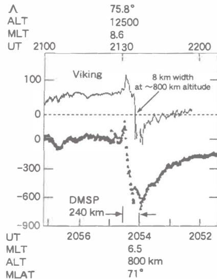
Fig. 3. Magnetic field traces from the Viking (top) and DMSP-F7 (bottom) satellites for the same event as Fig. 2 (adapted from Fig. 2 of Bythrow *et al.* (1987)). The spatial resolution (in invariant latitude) of the Viking data is one order of magnitude higher than the DMSP data.
