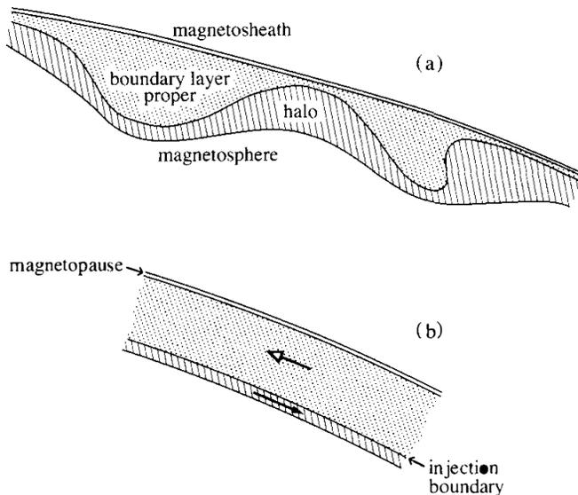
Fig. 12. (a) Schematic illustration of boundary layer plasmas based on the ISEE 1 and 2 satellite observations by Sckopke *et al.* (1981). (b) Simple model of the injection boundary, roughly parallel to the magnetopause boundary. The open- and closed-headed arrows denote antisunward and sunward plasma flows, respectively.
