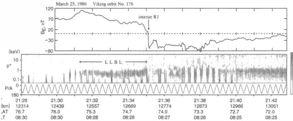
Fig. 2. Viking observations of the east-west component of the magnetic field (top), the energy-time spectrogram of positive ions (bottom), and the particle pitch angle with  $0^\circ$  denoting precipitating particles (very bottom) (adapted from Plate 1 of Potemra *et al.* (1987)). The ion spectrogram also shows ion conics characterized by the “tuning fork” signatures (Gurgiolo and Burch, 1982) beginning at about 2131:30 UT.
