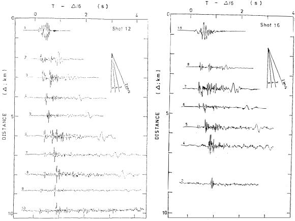
Fig. 2. Record section for Shot 12. Numerals are station numbers shown in Fig. 1.
