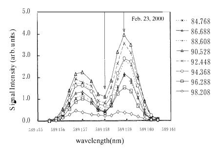
Fig 2. Backscatter signal intensity from the sodium  $D_2$  Doppler-broadened absorption spectrum. The arrows indicate the data used for the two-frequency method.
