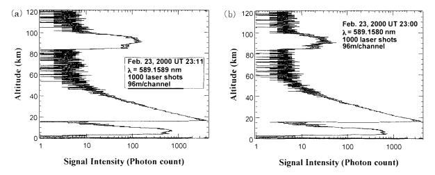
Fig. 1. Backscatter signal received by a photomultiplier. The laser wavelength was tuned (a) at  $\lambda = 589.1589$  nm near the sodium  $D_{2a}$  peak, and (b) at  $\lambda = 589.1580$  nm near the minimum between the  $D_{2a}$  and  $D_{2b}$  peaks.
