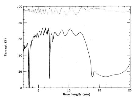
Fig. 5. Optical properties of TiO<sub>2</sub> mold film attached by a carbon mold film. Solid line indicates the transmission and dotted line the reflection.
