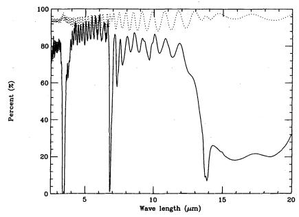
Fig. 4. Optical properties of TiO<sub>2</sub> mold film. Solid line indicates the transmission and dotted line the reflection.
