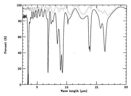
Fig. 3. Optical properties of BaSO<sub>4</sub> mold film. Solid line indicates the transmission and dotted line the reflection.
