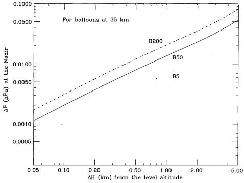
Fig. 2. The descend altitude form 35 km vs. the inner pressure at the nadir for three balloons; B5: 5000 m³, B50: 50000 m³, and B200: 200000 m³ in volume.
