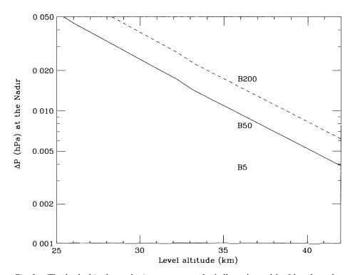
Fig. 3. The level altitude vs. the inner pressure of a balloon descend by 1 km from the level altitude for three balloons; B 5: 5000 m³, B 50: 50000 m³ and B 200: 200000 m³ in volume.
