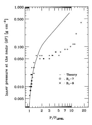
Fig. 4. Comparison of the theoretical curve on the inner pressure at the nadir of a balloon and experiments using balloons with volume of 1000 m³ (NISHIMURA et al., 1968). The vertical axis shows the inner pressure and the horizontal axis shows the atmospheric pressure P normalized by that at the level altitude P<sub>LEVEL</sub>. Theoretical curve well describes the experiments except at large P/P<sub>LEVEL</sub>.
