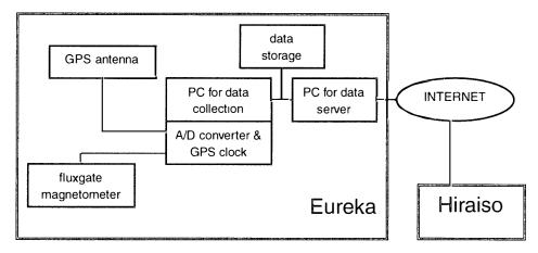
Fig. 3. Schematic diagram of the real-time geomagnetic field monitoring system.
