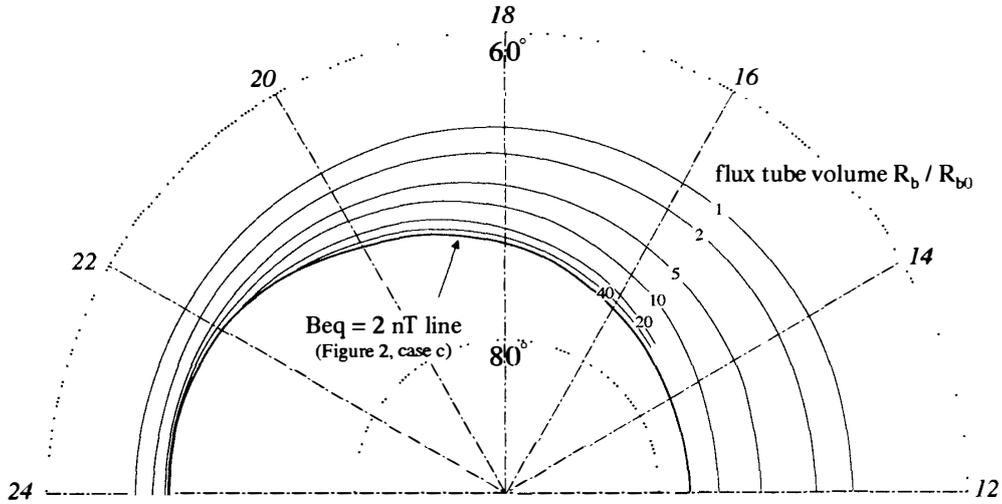
Fig. 7. Equicontours of the flux tube volume  $R_b$ , normalized by  $R_{b0}$  (for their definitions, see text), on the ionospheric plane. Superposed is the  $B_{eq}=2\text{ nT}$  line (in Fig. 2, case c).
