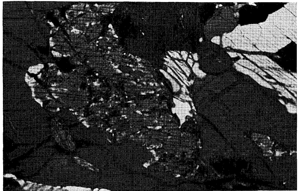
Fig. 28. Clinopyroxene altered to hornblende in clinopyroxene syenite gneiss ( \times 70 ).
