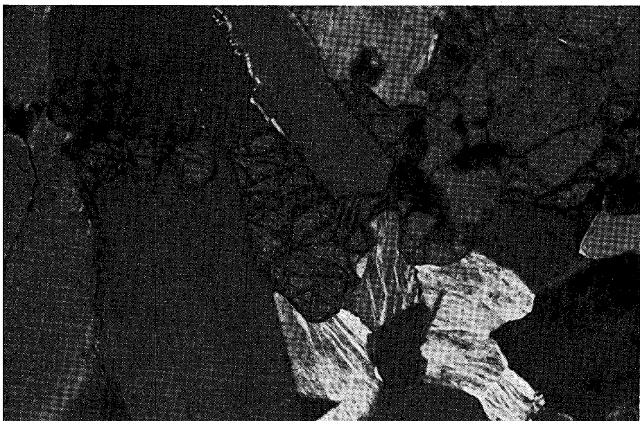
Fig. 32. Biotite associated with sphene in clinopyroxene quartz syenite gneiss ( \times 70 ).
