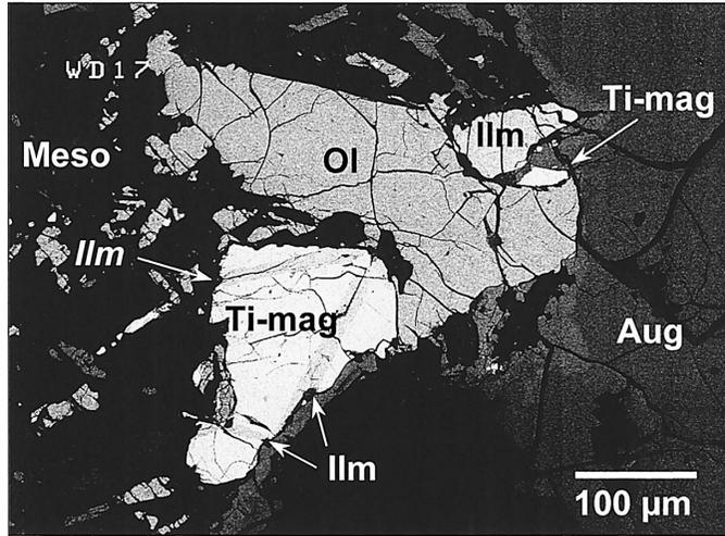
Fig. 12. BSE image of the mesostasis area including opaque minerals in Y000593. Ti-rich magnetite grain in this image shows ilmenite exsolution lamellae parallel to three orientations (probably parallel to (111)). An individual ilmenite grain is also present. Ti-mag: Ti-rich magnetite. Ilm: ilmenite. Ol: olivine. Aug: augite. Meso: mesostasis.
