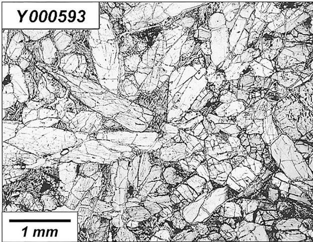
Fig. 1a. Optical photomicrograph (open nikol) of the Y000593 thin section (Y000593,68-1). The thin section shows a cumulate texture mainly composed of augite, olivine and the mesostasis. Augite shows a prismatic crystal texture up to 1.5 mm long.
