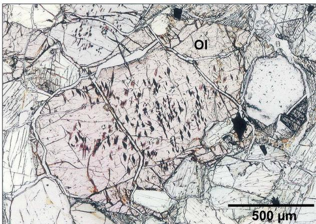
Fig. 2b. Optical photomicrograph (open nikol) of an altered olivine grain in Y000593. The presence of brown alteration products along the fractures is remarkable in this olivine grain. This olivine grain contains a poikilitic augite grain (Aug-p). The mesostasis (Meso) is also showing alteration similar to olivine. Ol: olivine. Aug: augite.
