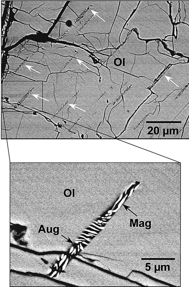
Fig. 8a. BSE images of an olivine grain in Y000593 including abundant symplectic inclusions (indicated white arrows in the above image). These symplectic inclusions are composed of augite (dark area) and magnetite (bright area). Ol: olivine. Aug: augite. Mag: magnetite.
