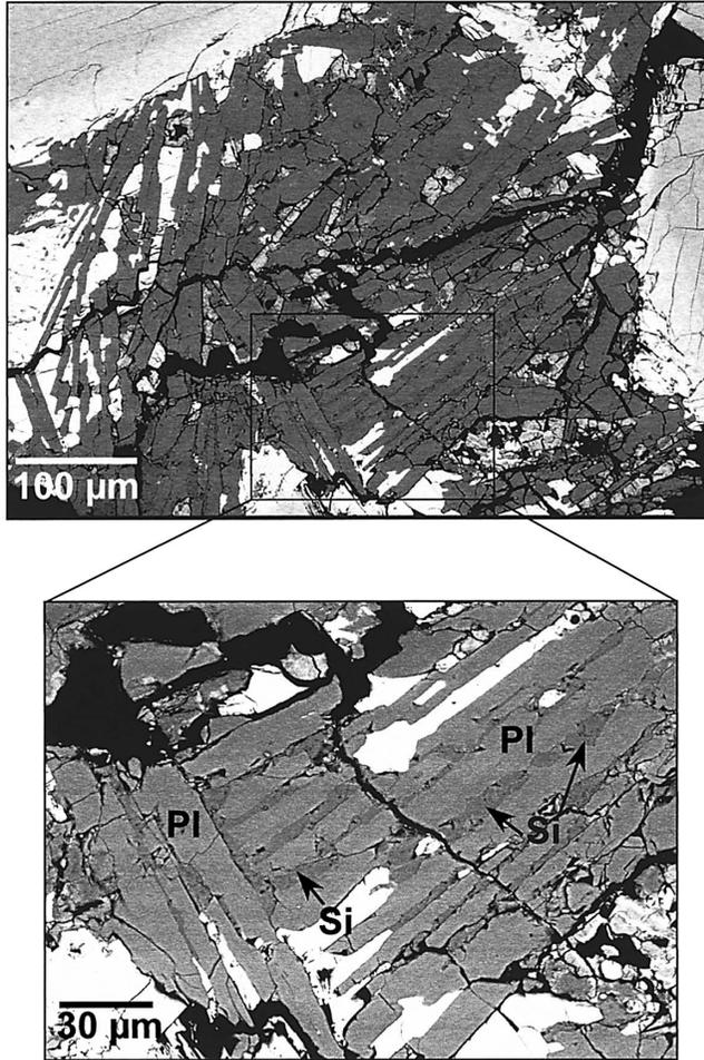
Fig. 9. BSE images of the mesostasis area in Y000593. The mesostasis is mainly composed of lath-shaped plagioclase (Pl) intergrown with silica (Si). Bright lath-shaped grains in the mesostasis are olivine and pyroxene.
