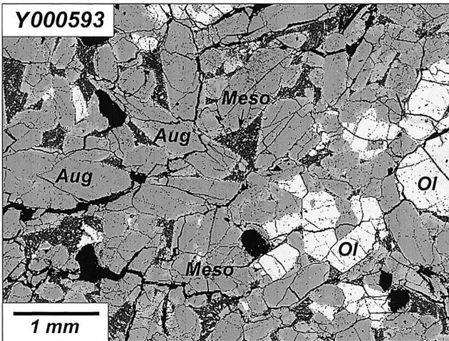
Fig. 1b. Back-scattered electron (BSE) image of the same field of view as Fig. 1a. Bright phases are mostly olivines. Augite is principally homogeneous except for the rims adjacent to the mesostasis. Aug: augite. Ol: olivine. Meso: mesostasis.
