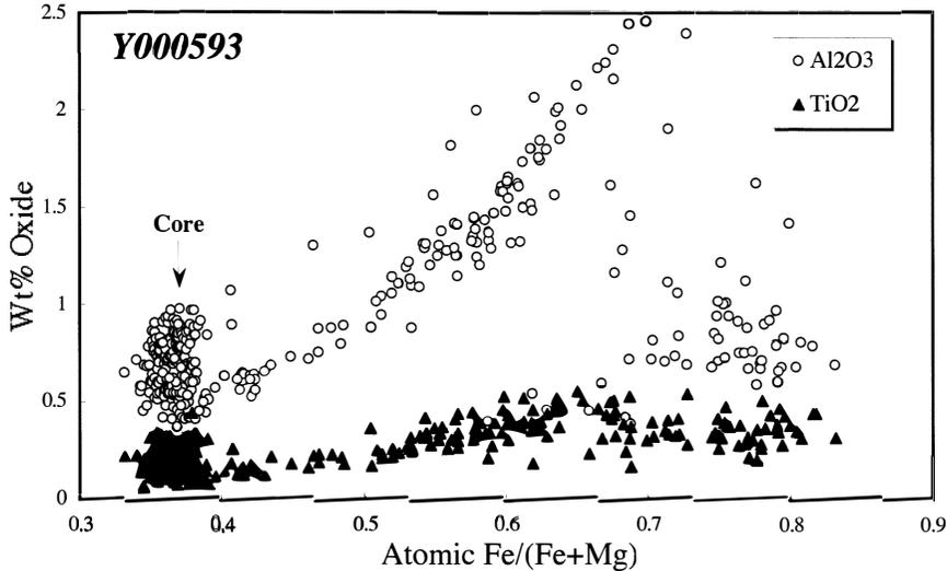
Fig. 6. Al and Ti variations of augites in Y000593 versus the *fe#* variation. Al shows the compositional range of  $Al_2O_3=0.4-1.0$  wt% in the core, and then increases as *fe#* increases. The most Fe-rich augite has lower Al contents ( $Al_2O_3=0.5-1.0$  wt%). The Ti content also has a cluster in the core ( $TiO_2=0.1-0.3$  wt%) and then shows a similar behavior to Al. Ti increases as *fe#* increase, but it slightly decreases when *fe#* reaches 0.65.
