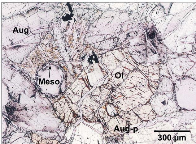
Fig. 2c Optical photomicrograph (open nikol) of the mesostasis area in Y000593. Note the presence of brown alteration products interstitial to plagioclase laths. The mesostasis includes a Ti-rich magnetite grain (Ti-mag). Some of the tiny opaque grains in the mesostasis are Fe sulfide. Aug: augite. Ol: olivine.
