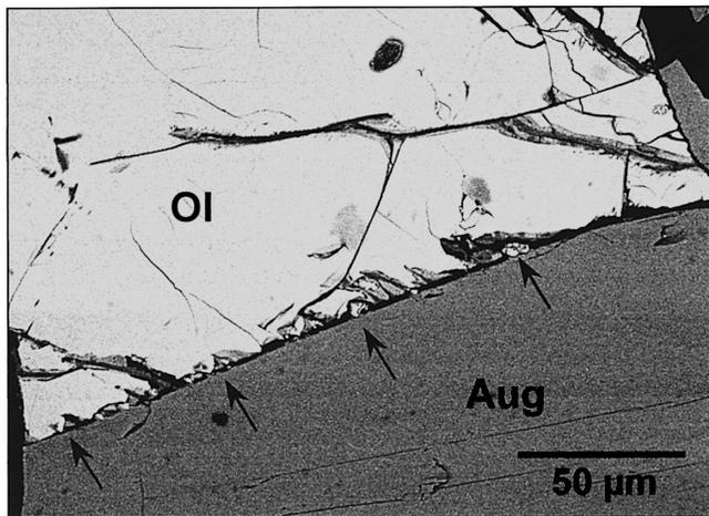
Fig. 8d. BSE image showing the patches with symplectic textures along the grain boundaries between poikilitic augite (Aug) and the host olivine grain (Ol) in Y000593.
