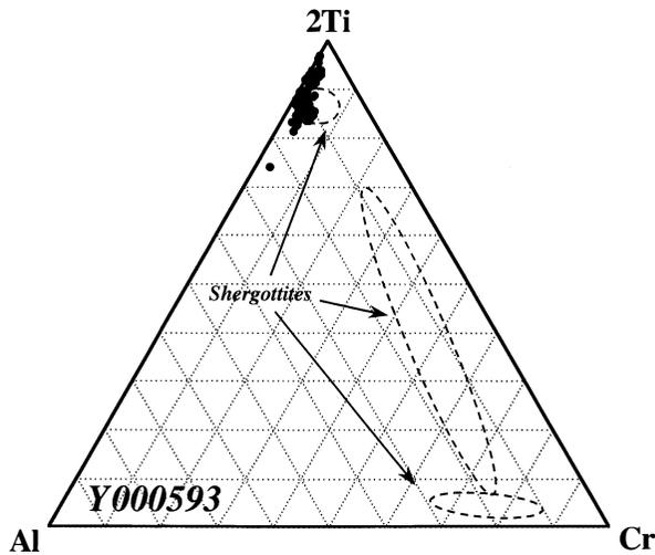
Fig. 11. Major element compositions (Cr, Al and Ti) of spinels in Y000593. Spinels in Y000593 are Ti-rich magnetite (ulvöspinel). The dashed circles show the compositions of spinels in shergottites, which are quite different from those of Y000593.
