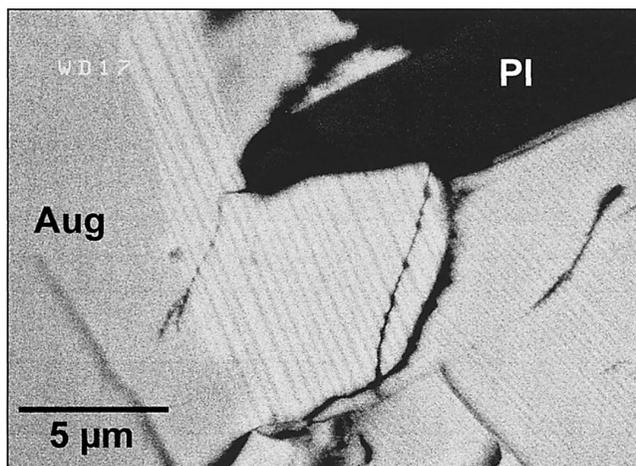
Fig. 4c. High resolution BSE image of Fe-rich pyroxenes at the cumulus pyroxene rims. Fine exsolution texture (thinner than  $500\mu\text{m}$  wide) is clearly observed. Probably, darker lamellae correspond to Ca-rich pyroxene and brighter ones are Ca-poor pyroxene. Aug: augite. Pl: plagioclase in the mesostasis.
