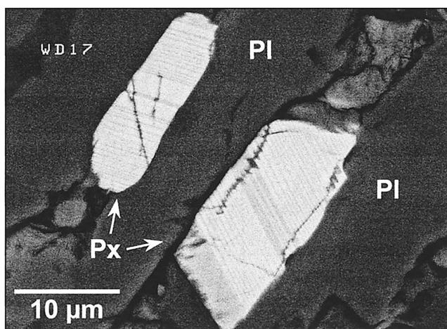
Fig. 4d. High resolution BSE image of Fe-rich pyroxenes in the mesostasis. These two pyroxene grains also show the presence of fine exsolution lamellae of similar size to that at the pyroxene edges (Fig. 4c). Px: Fe-rich pyroxene in the mesostasis. Pl: plagioclase in the mesostasis.
