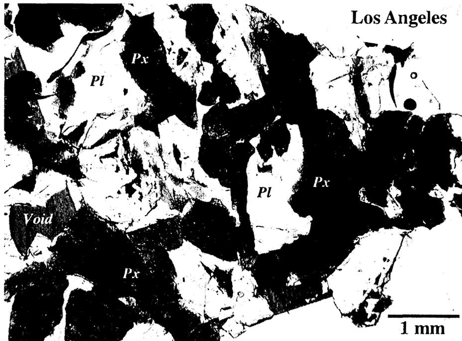
Fig. 1. Photomicrograph of Los Angeles. The scale bar is 1 mm. Pyroxenes (Px) show dark appearance, probably due to shock. Plagioclases (Pl) are transformed into amorphous states ("maskelynites").
