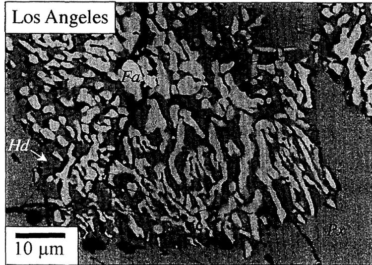
Fig. 3. BSE images of hedenbergite-fayalite-silica assemblages of Los Angeles, showing complex dendritic textures. They are usually associated with ulvöspinel, Ca phosphates, or some other late-crystallization phases. Sp: ulvöspinel. Ilm: ilmenite. Hd: hedenbergite. Fa: fayalite. Si: silica. Px: pyroxene.
