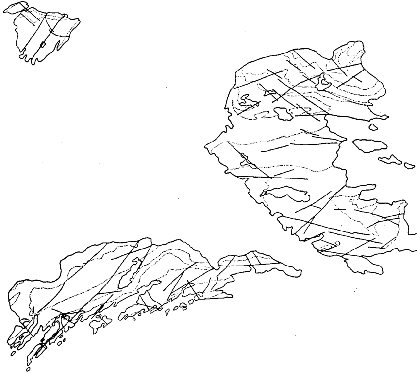
Fig. 4. Distribution of fractures traced from aerial photographs. Solid line: fractures, Dotted line: boundary of geologic bodies.
