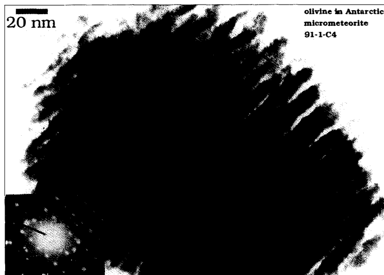
Fig. 10. A TEM image of a typical altered olivine grain in particle 91-1-C4. These olivine grains contain planar channels parallel to (001) plane. Selected area electron diffraction (SAED) pattern shows that diffraction spots have streaks parallel to c^* of olivine due to the planar channels. Some diffraction spots from the adjacent grains are also shown in the SAED pattern, because the selected area aperture used here could not exclude diffraction from other grains. It is thought that terrestrial weathering proceeded along (001).
