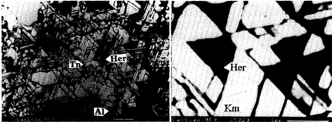
Fig. 1. Back-scattered electron (BSE) image of the texture of a hercynite-kamacite aggregate. Km—kamacite, Her—hercynite, Tn—taenite; Al—corundum; gray—iron oxides.
