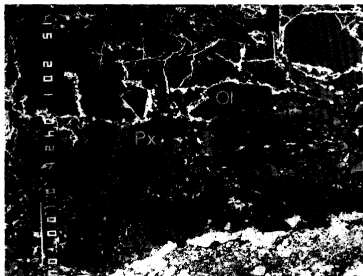
Fig. 5. A part of the pyroxene layer in C#1. Ca-poor pyroxene is usually mantled by Ca-rich pyroxene, and both of them are closely in contact with plagioclase and olivine of the host. The thin bright rims along boundaries and/or cracks of plagioclase and olivine are hedenbergite (Hed). The width is 590 \mu\text{m} .
