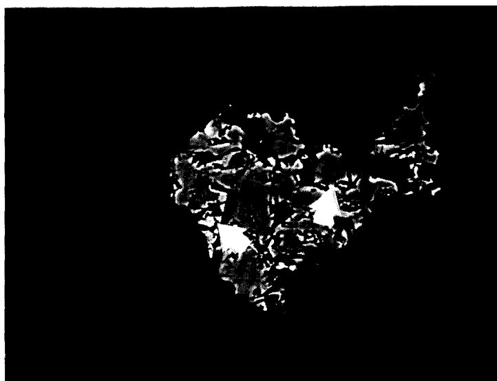
Fig. 7. A BSE image of a pyrrhotite grain. Brighter portions (indicated by arrows) are seen within gray host pyrrhotite, where Ni concentration is fairly high up to 25 wt%.
