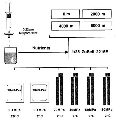
Fig. 1. A schematic representation of incubation. All the samples collected were put into sterile polyethylene bags, supplied with sterile nutrients and incubated under six different conditions (0.1 MPa/2°C, 0.1 MPa/2°C, 20 MPa/2°C, 40 MPa/2°C, 60 MPa/2°C and 80 MPa/2°C). All incubation was done simultaneously in the dark.
