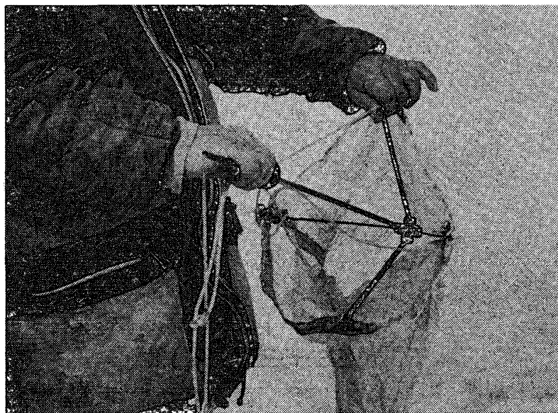
Fig. 2. Photograph of the umbrella net with the mouth open. Note the four hinged arms.
