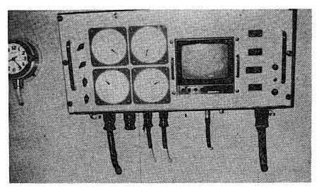
Fig. 4. Data output terminal of ship's navigation information.
