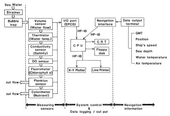
Fig. 1. A block diagram of the surface water monitoring system installed on board the icebreaker SHIRASE.
