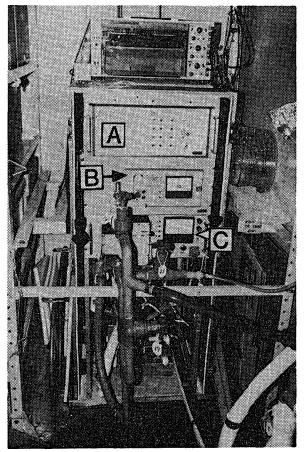
Fig. 2. A rack of measuring sensors of the monitoring system. A: I|O port (EPCS; Electronic plankton counting and sizing system), B: DO meter, and C: Turner Designs fluorometer.
