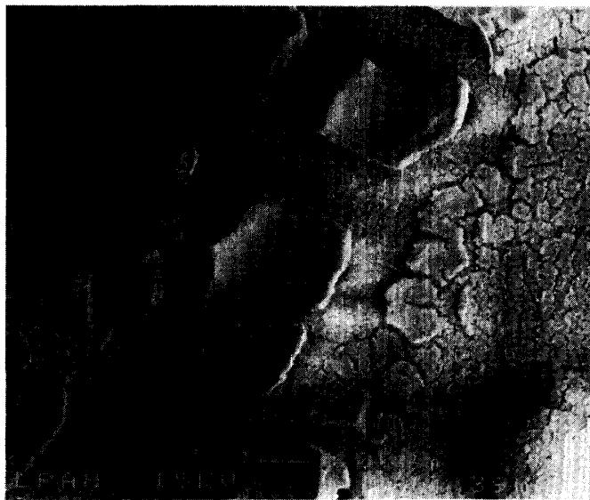
Fig. 8. SEM photograph of the surface of the alteration products layer developed on the glass after 8 days alteration in \text{H}_2\text{SO}_4 solution with pH1 at 80°C (scale bar=100 \mu\text{m} ).
