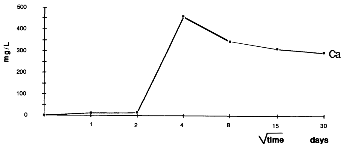
Fig. 3. Calcium content evolution in solution versus time, for H_2SO_4 solution with pH 4 at 80°C.
