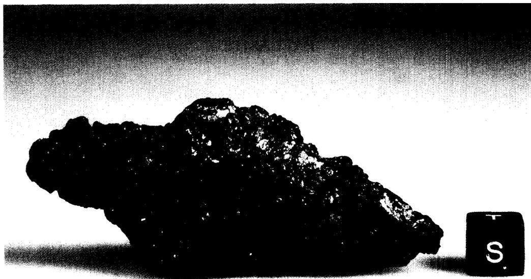
Fig. 1. Yamato-8451 meteorite is an arrowhead-shaped specimen, weighing 54.8 g, partly covered by fusion crust and showing brownish-black weathered Fe-Ni metal and light brownish silicates (mostly olivine grains). The scale of the cube is 1 cm.
