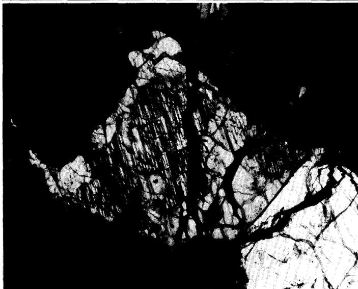
Fig. 4b. Photomicrographs of three different coexisting pyroxenes, 1 mm across. Polysynthetic twinned exceptionally Ca-poor Opx (Opx-1, core) is mantled by non-polysynthetic Opx (Opx-2, rim). Clinopyroxene (Cpx) is included in non-polysynthetic Opx (right bottom). This photo corresponds to the elemental map (Fig. 5). The field of view is 1.6 mm. Crossed polars.
