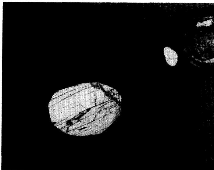
Fig. 4d. Clinopyroxene (Cpx) crystal in Ca-poor Opx (Opx-2, non-polysynthetic), 150–200  $\mu\text{m}$ .
