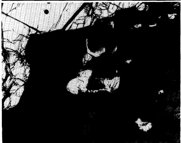
*Fig. 3c. Very small olivine crystals (Ol) coexist with Ca-poor Opx (Opx-2, non-polysynthetic twinned). The olivine crystal is 50–150  $\mu\text{m}$  across. Crossed polars.*
