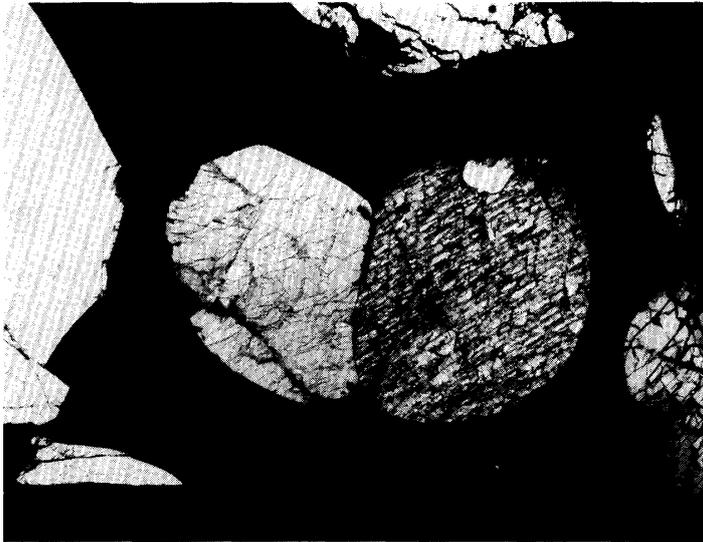
Fig. 4a. Well rounded exceptionally Ca-poor Opx (Opx-1, right), 1.6×2.0 mm and sub-angular olivine (left), 1.4×1.6 mm, in Fe-Ni metal (black). Orthopyroxene shows typical polysynthetic twinning, and includes olivine (white on top, 0.3 mm). Crossed polars.
