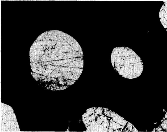
*Fig. 3a. Well-rounded olivine grains, 1 to 1.4 mm across, set in the metal matrix. Plane polarized light.*
