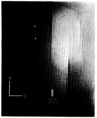
Fig. 3. An EM image of voids in B-7904. (020) lattice fringes of 5 A are found.
