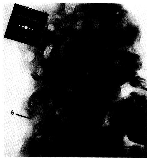
Fig. 2. An EM image of typical void structure in olivine in B-7904. Many voids are crystallographically controlled in shape.
