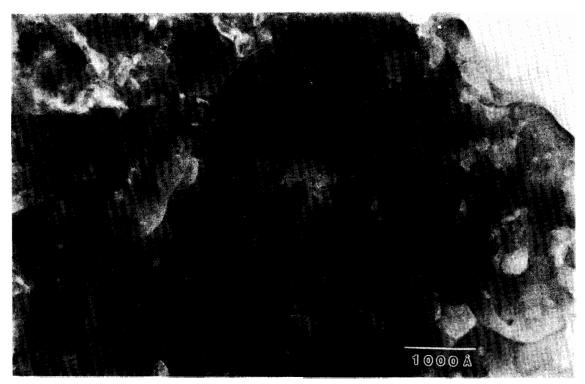
Fig. 4. EM image of matrix in B-7904, showing very frequent voids or bubbles.
