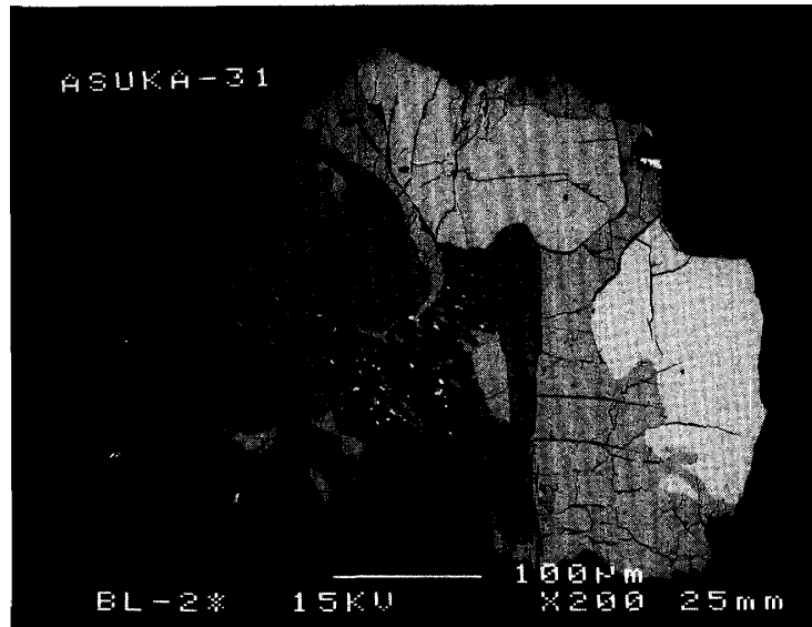
Fig. 4a. Back-scatter electron (BSE) image of sample A31-BL2: Coarse-grained mesostasis consisting of fayalite (gray), ulvöspinel (light gray), ilmenite (light gray), apatite (gray, center and upper left), plagioclase (darker gray), and silica (dark gray). Bright specks are Fe-sulfides.
