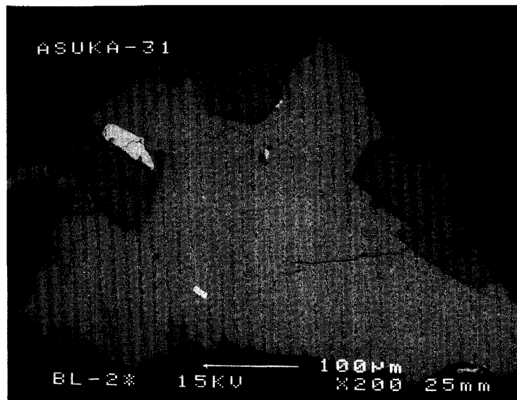
Fig. 4b. Back-scatter electron (BSE) image of sample A31-BL2: Ulvöspinel grain containing ilmenite (gray), Fe-sulfide (white, large), Ni-poor metal (white, small), and titaniferous fayalite (between ilmenite and ulvöspinel).
