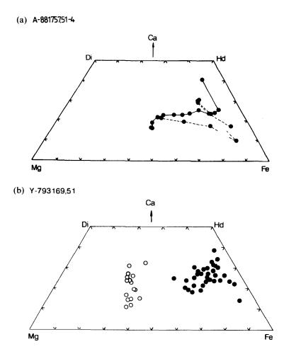
Fig. 4. (a) Pyroxene quadrilateral of A-881757 (present study), showing more Fe-rich trend than that of Y-793169. The circles connected by lines represent one traverse.
