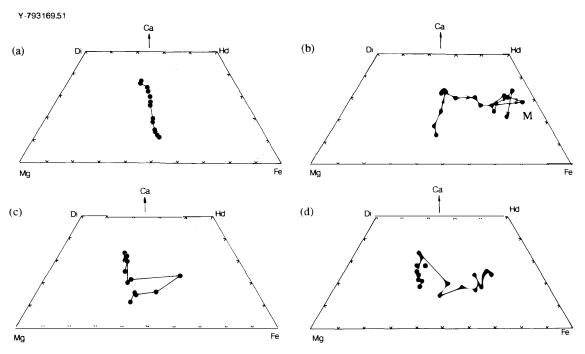
Fig. 2. Pyroxene quadrilaterals of Y-793169, showing chemical variations of some typical zoning trends. Subnumbers (a-d) refer to different single crystals. M: Mesostasis
