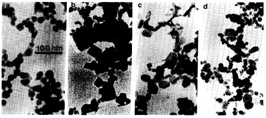
Fig. 5. Typical EM image of iron oxide particles (a) FeO (wüstite). (b)  $Fe_3O_4$  (magnetite). (c)  $\alpha$ -Fe<sub>2</sub>O<sub>3</sub> (hematite). (d)  $\gamma$ -Fe<sub>2</sub>O<sub>3</sub> (maghemite).
