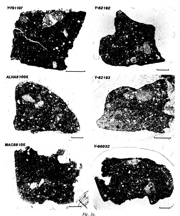
Figs. 2a, b. Photomicrographs of thin sections of each lunar meteorite (plane-polarized light), except Y-793169(b) and Asuka-31(b) which is in cross-polars, showing the maskelynitized plagioclase. Scale bars are 0.2 mm.
