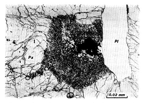
Fig. 4. Photomicrograph of symplectite in Asuka-31. Troilite (black) rimmed by olivine is surrounded by symplectite halo. Symplectite shows the worm-like texture composed mainly of an olivine-pyroxene-plagioclase intergrowth. Pl (plagioclase : anorthite), Px (pyroxene).
