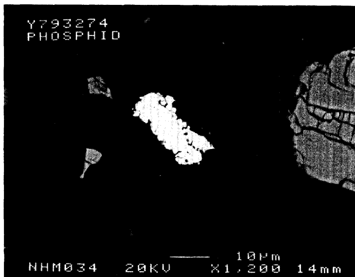
Fig. 15. BSE image of a grain (light gray, center) of the mineral barringerite, (Fe,Ni)_2P , in sample ,94. This is the first time this mineral is found in lunar rocks (see BRAND-STÄTTER et al. , 1991).
