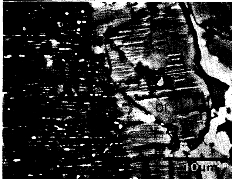
Fig. 2. BEI of a mineral fragment of olivine. The dark, left side of the olivine is the reduced zone consisting of olivine, metallic Fe blebs and SiO 2 mineral. The right-hand side is a poorly reduced zone.
