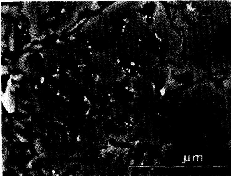
Fig. 4b. An enlarged view of (a). Metallic Fe grains (Fe) are dispersed in and around olivine grains (Ol).
