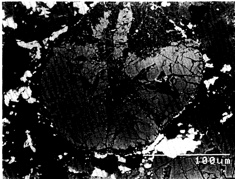
Fig. 10. BEI of two large pyroxene chondrules. In both (a) and (b), the large orthopyroxene (Opx) phenocrysts in glass have the ferrous core and the Ca-rich rim. (a) and (b) correspond to (F-1) and (F-2) in the text.
