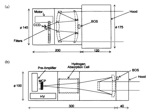
Fig. 1. Schematic drawings of (a) UPI-TVIS and (b) UPI-TUV. Scales are in mm.
