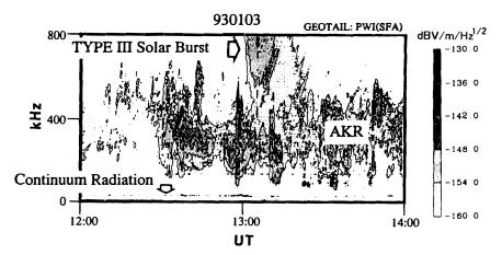
Fig. 1. Dynamic spectra of AKR electric field observed with Sweep Frequency Analyzer onboard GEOTAIL spacecraft on 3 January 1993.
