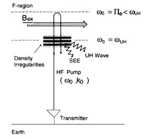
Fig. 1. Schematic of the typical ionospheric heating situation.
