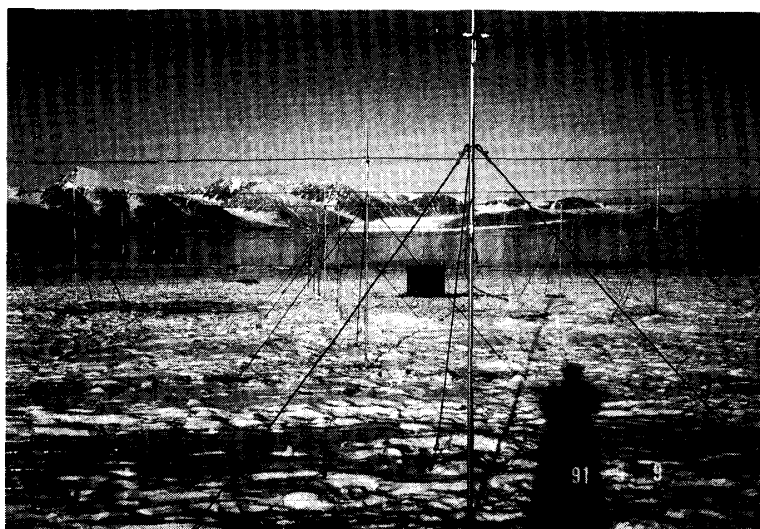
Fig. 1. A portion of the 64-dipole phased array installed at Ny-Alesund. The phasing/receiver box is located at the center of the array.
