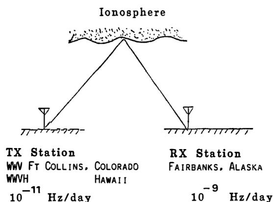
Fig. 1. HF Doppler measurement system.
