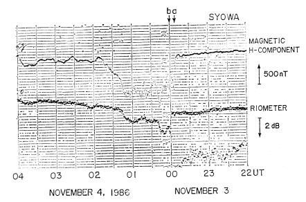
Fig. 4. Negative change in the magnetic H-component starting at the time of SSC (denoted with a) and the CNA observed with the conventional broad beam riometer (b) starting 7 min later than the onset of SSC.
