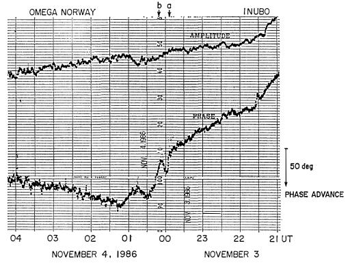
Fig. 5. Phase and amplitude variations of the Omega Norway signal as received at Inubo, Japan. The phase advanced simultaneously with the SSC (denoted with a), while the phase advance associated with the substorm is delayed by about 6 min from the onset of the substorm in the midnight (b).
