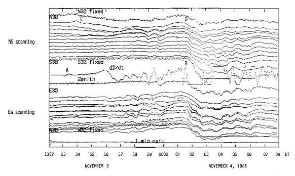
Fig. 2. Cosmic noise absorptions associated with a storm sudden commencement (denoted by C in the figure) and substorm (D), observed by the north-south and east-west scanning beams. The onsets of the SSC and substorm are indicated with A and B by the curve of ULF D-component (dD/dt).
