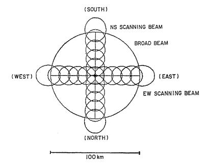
Fig. 1. Field of view at the ionospheric height (90 km) of the scanning beam (small circles) and conventional broad beam (large circle). Two scanning beams cover a range of about 120 km in the north-south and east-west directions with a spatial resolution of 10 km.
