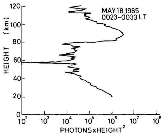
Fig. 1. Realtime displayed data of height vs. photon signals  $\times$  squared height obtained by accumulating the returns from 100 laser shots.
