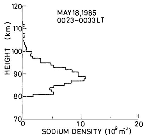
Fig. 2. Vertical profile of the sodium density calculated from the data shown in Fig. 1.
