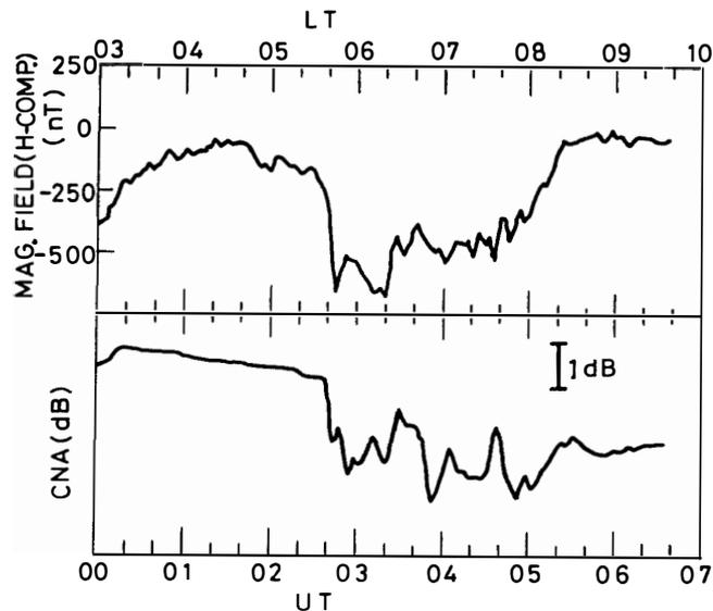
Fig. 13. Time variations in geomagnetic field  $H$ -component and cosmic noise absorption (CNA) on June 1, 1985.
