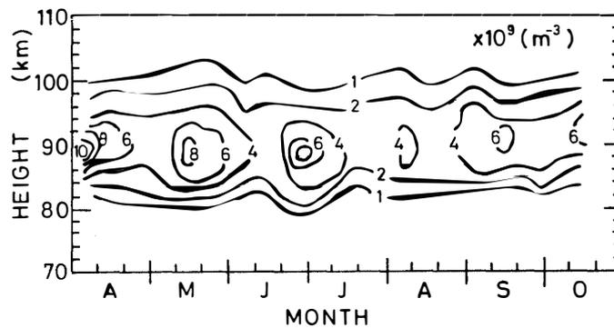
Fig. 4. Semiseasonal variation in nightly average vertical sodium density profile in the form of a contour plot from April to October, 1985.
