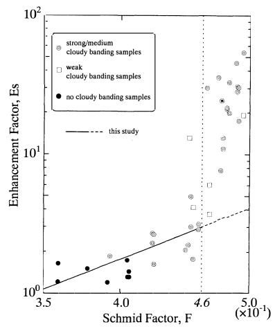
Fig. 3. A log-log plot of Schmid factors and enhancement factors. Each data point indicates light scattering intensity of a cloudy band in the slab samples.
