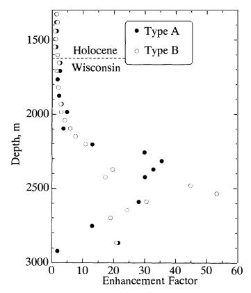
Fig. 2. The profile of enhancement factor from the uniaxial compression tests.
