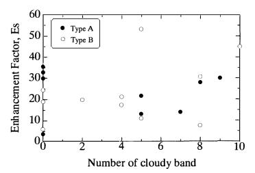
Fig. 4. Enhancement factors versus the number of cloudy bands in the uniaxial compression test specimen for Schmid factors lager than 0.46. The solid circles and open circles are Type A and Type B uniaxial compression test conditions, respectively.
