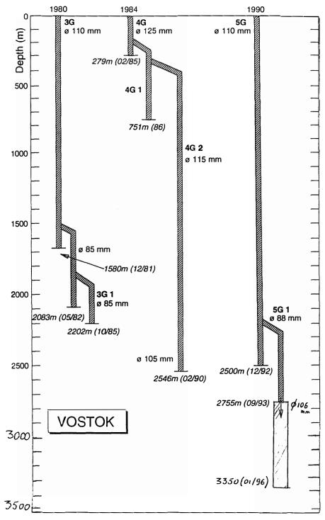
Fig. 2. Vostok drilling has been a long-term effort of Russian glaciologists. Several successive bore holes have been necessary before reaching the present depth of 3250 m.
